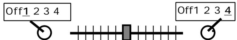
"Hard left" selects the channel set up of the **Assign Left** knob. In this example, it is Channel 1. "Hard right" selects the channel set up on the **Assign Right** knob. In this example, it is Channel 4. With the crossfader centered, both assigned channels are live. Use the crossfader for fast and seamless segues from one selected channel to the other. To turn off the crossfader simply turn both knobs all the way to the left.
